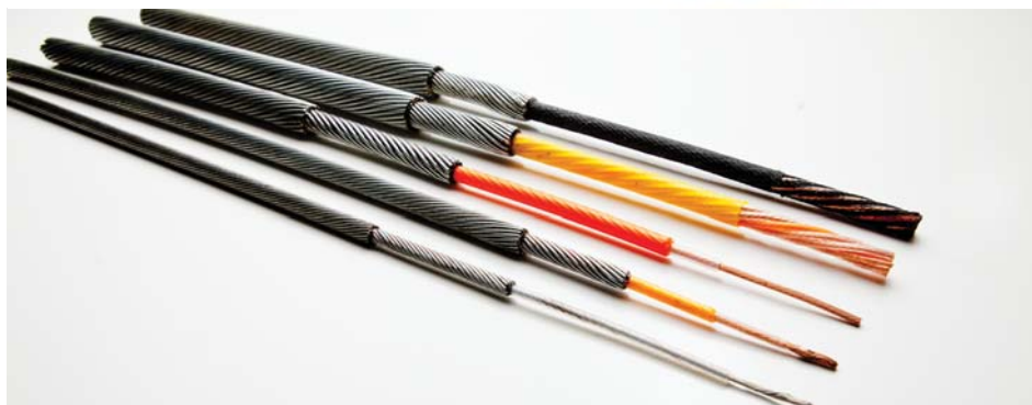
EMC are complex cables with a central copper conductor armored with special galvanized improved plow steel wires or special alloy wires. The cross-section shows DuraSlam, an EMC which is designed to resist drum crush (aka cable crush).
